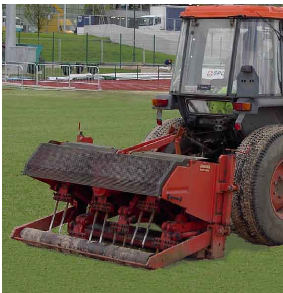
Specialist equipment such as a verti-drainer can be hired to maintain pitch quality
